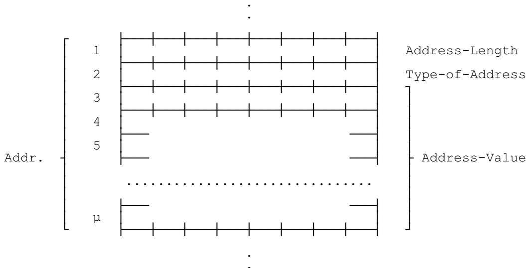
The Address-Length field is an integer representation of the number of useful semi-octets within the Address-Value field, i.e. excludes any semi octet containing only fill bits.
