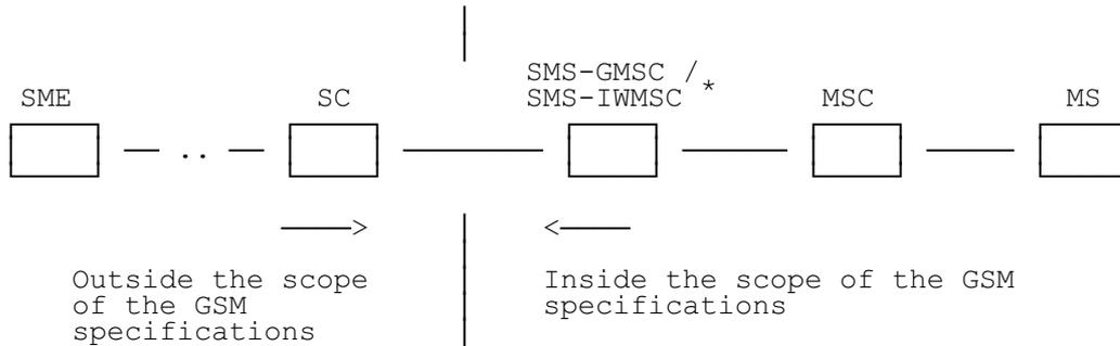
\*) : SMS-GMSC when the short message is transferred from the SC to the MS, SMS-IWMSC when the short message is transferred from the MS to the SC. The SC may be integrated with the SMS-GMSC/SMS-IWMSC.
