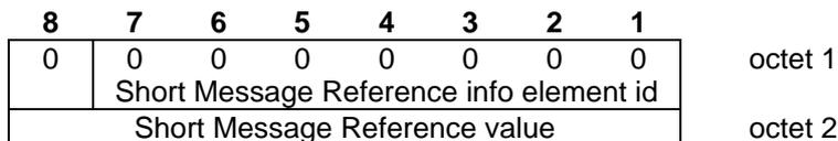
Figure 2.5.2/GSM 07.05: Short Message Reference information element
