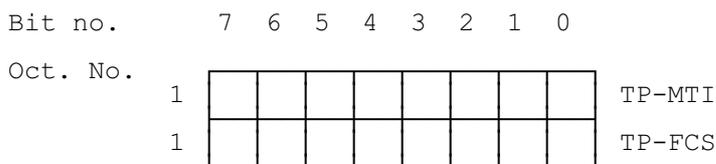
Bits 7 - 2 in octet 1 are presently unused and the sender shall set them to zero. If any of these bits is non-zero, the receiver shall not examine the other field and shall treat the TP-Failure-Cause as "Unspecified error cause".
