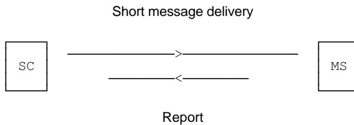
Figure 03.40/1: The Short Message Service mobile terminated, point-to-point.
