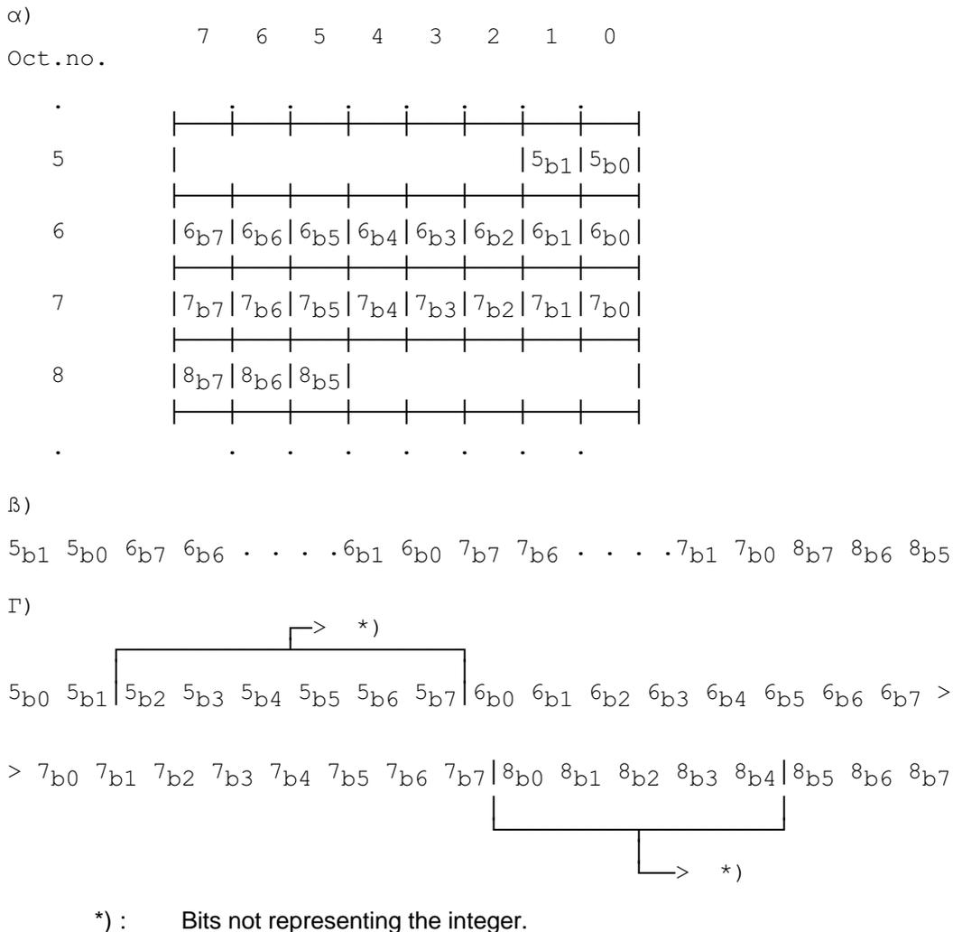
**Figure 03.40/8: 21 bits from the octets 5, 6, 7, and 8 in a short message α) will represent an integer as shown in β), and will be transmitted in an order as shown in Γ).**
