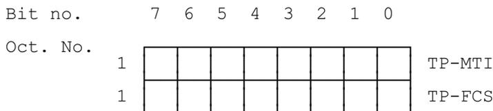
Bits 7 - 2 in octet 1 are presently unused and the sender shall set them to zero. If any of these bits is non-zero, the receiver shall not examine the other field and shall treat the TP-Failure-Cause as "Unspecified error cause".
