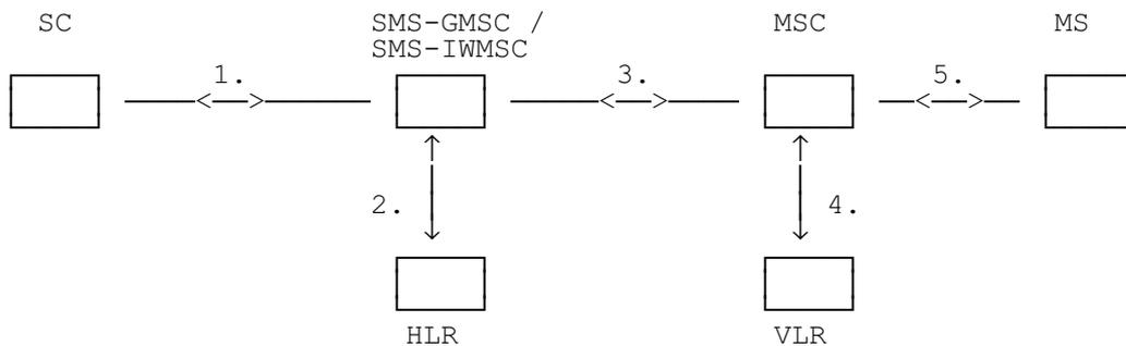
**Figure 03.40/5: The main network structure serving as a basis for the short message transfer.**
